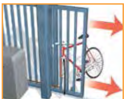
entrapment detection reverses gate when obstructed
