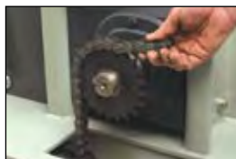
no slip chain drive #100 roller chain
