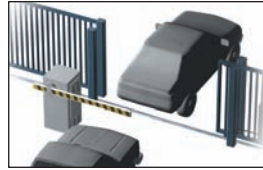
automatic p.a.m.s. sequencing with slide and swing gates
