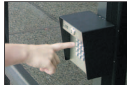
keypad User's enter their 4-5 digit unique PIN (personal identification number) to gain entry
