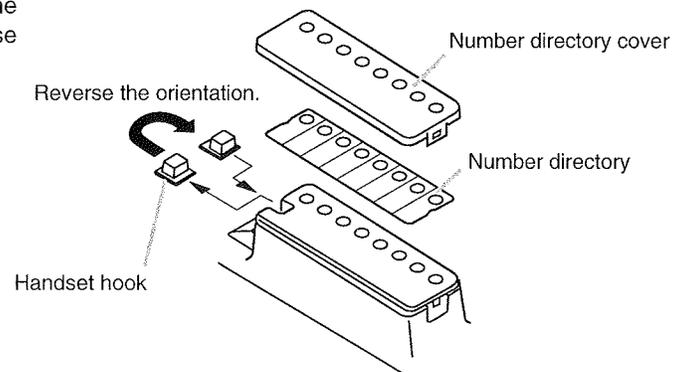
**Step 3.** After replacing the directory on the station, hook the directory cover's forward tab and push on the upper part of the directory cover.
