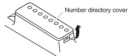
**Step 2.** Remove both the number directory cover and the directory. Remove the handset hook and reverse its orientation, then replace.
