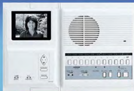
MYH-CUB Video Monitor, semi-flush mount
